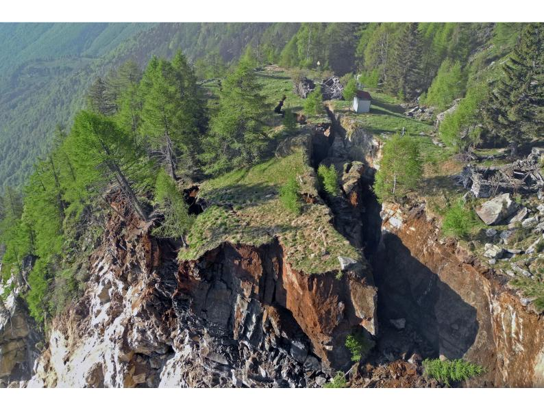
During the night of 14 May this year, 300,000 m3 (392,000 yd3) of rock broke off the Valegion mountain and crashed down 1,000 m (3,281 ft) to the valley floor in the Swiss canton of Ticino, near the village of Preonzo. Thanks in part to Leica Geosystems' Deformation Monitoring solution GeoMoS local authorities were able to evacuate the valley's industrial zone and to close the A2 highway and several cantonal roads at an early stage.
