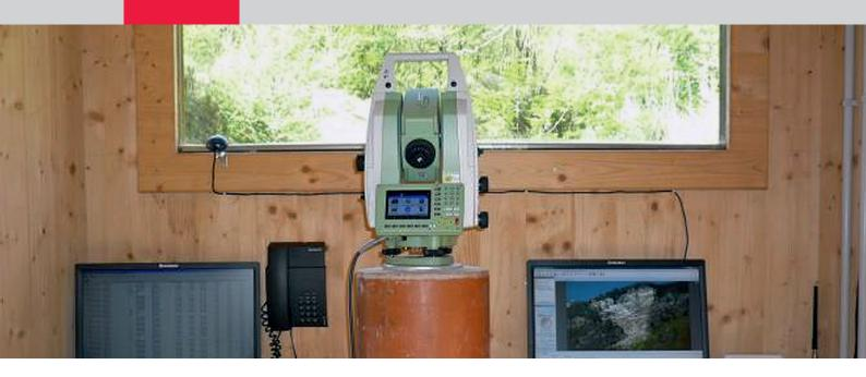
data with millimeter-accuracy in real-time, knowing when movements took place and in which direction. The responsible experts were able to analyze developments and trends, and combined this data with additional information. The complete measurement history is very valuable to the geologists' further analysis."
